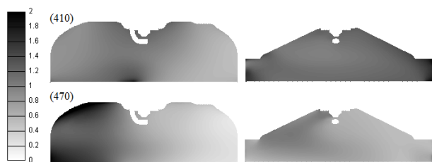
Fig. 19 Equivalence ratio of in-cylinder charge at ignition timing for SOI 410° CA and 470° CA
