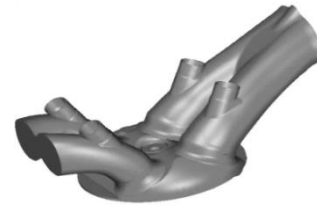
Fig. 9 A simulated model of cylinder head of EF7 engine
